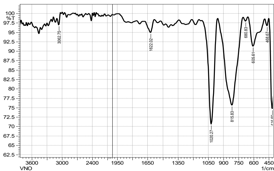
Figure 3. presents the Fourier-transform infrared (FTIR) spectrum of vanadium pentoxide ( V_2O_5 ).
